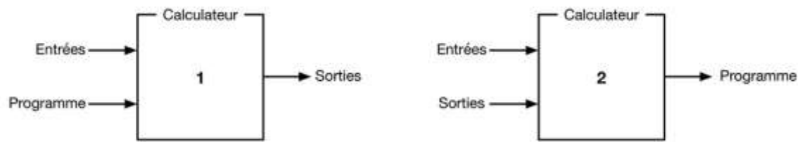
Figure 1 Machine hypothético-déductive (1) et machine inductive (2)
